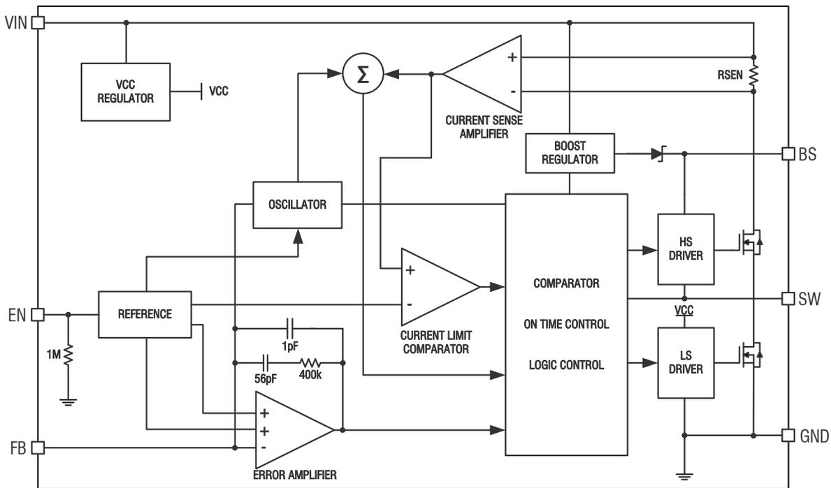
Figure 2. MT1470 Block Diagram
