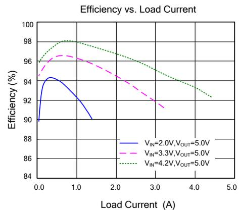
Figure 2. Efficiency Figure
