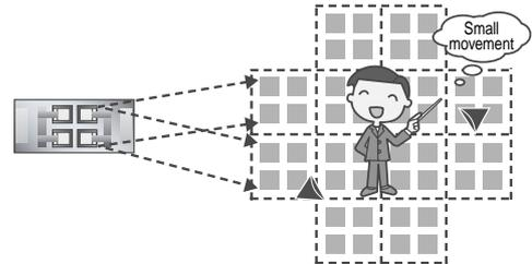
4. Small temperature differences also detected. N a P i O n detects the temperature difference between the detection target and its surroundings, and the lowest required temperature difference to the background is 4°C 7.2°F.
