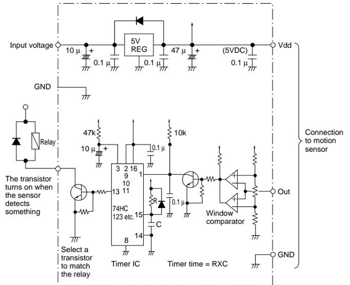
Note: This is the reference circuit which drives the MP motion sensor. Install a noise filter for applications requiring enhanced detection reliability and noise withstanding capability.
