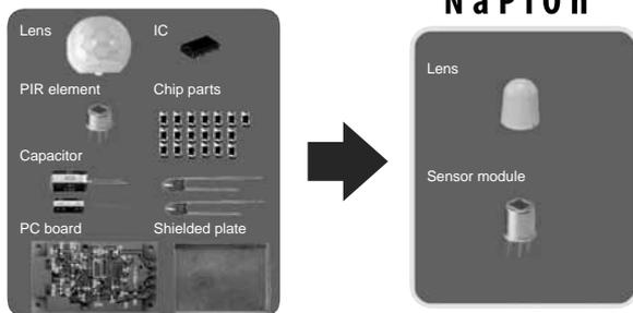
2. Ideal for small-movement detection thanks to quad-type pyroelectric element. The quad-type pyroelectric element contained in N a P i O n has four receptors. Since the detection zone within the detection range is so precise, even small movements can be detected.
