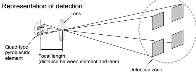
3. Lenses can be miniaturized because the pyroelectric element is small. A short focal length is all that's required even when detecting at the same distance, because the size of the N a P i O n pyroelectric element is so small. This means that high precision is maintained even though the lens is small and the sensor itself has been miniaturized.
