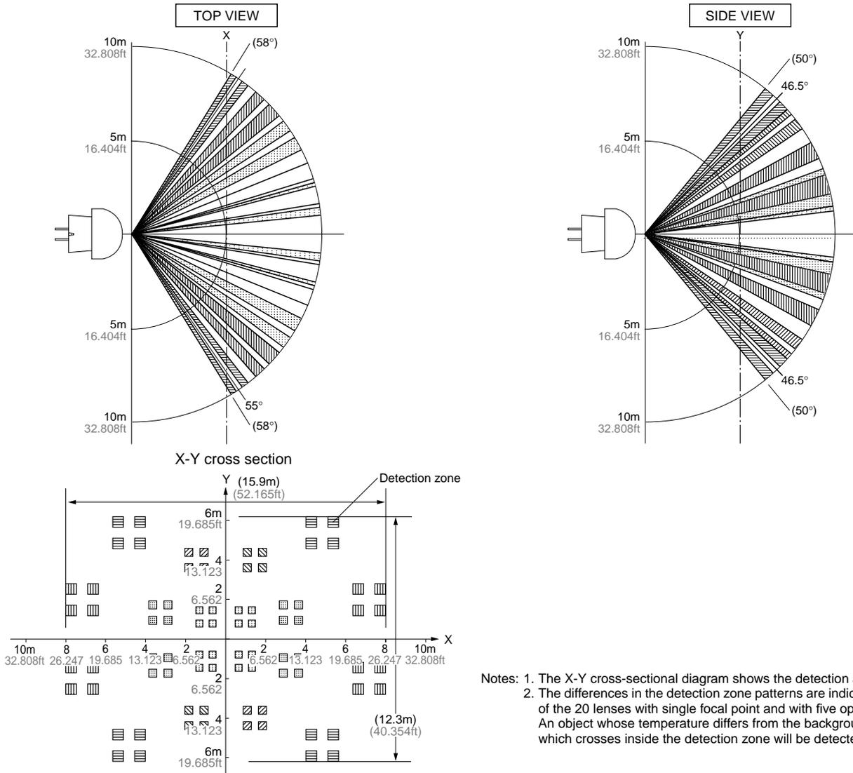
Notes: 1. The X-Y cross-sectional diagram shows the detection area.
