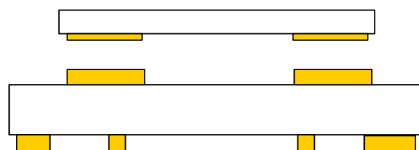
Figure 19. Correct PCB Top Metal Pattern Under Package
