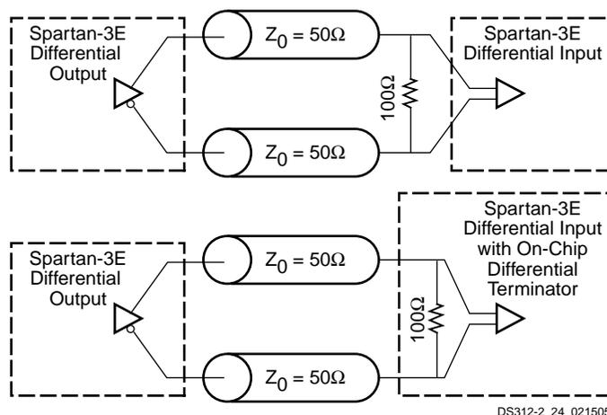
Figure 8: Differential Inputs and Outputs
