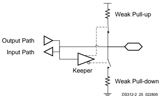
Figure 9: Keeper Circuit
