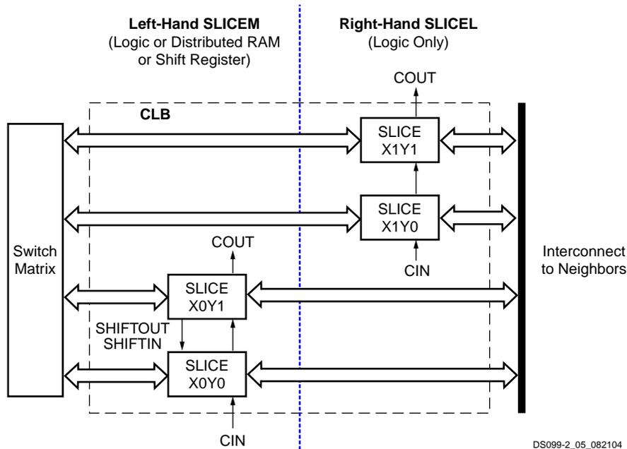
Figure 13: Arrangement of Slices within the CLB
