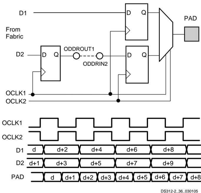
Figure 7: Output DDR Using Spartan-3E Cascade Feature
