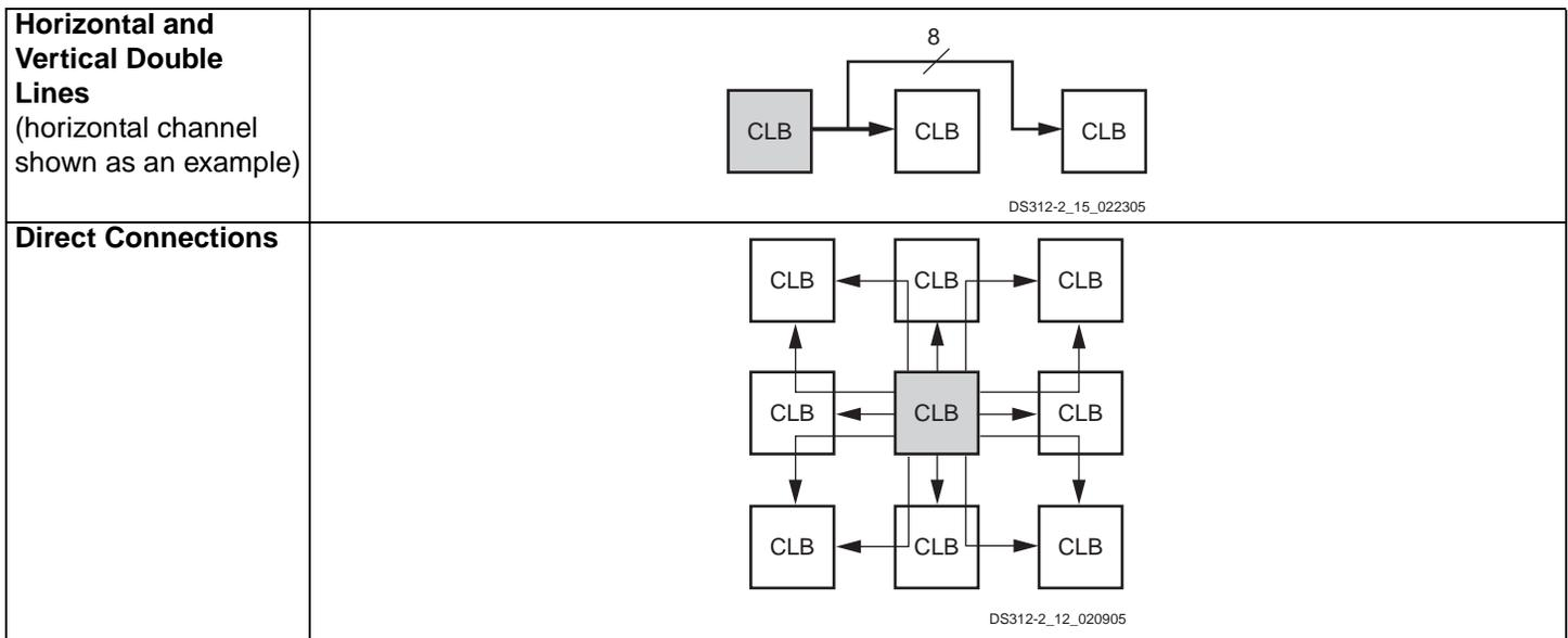
Figure 47: Interconnect Types between Two Adjacent Interconnect Tiles
