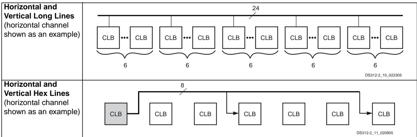
Figure 47: Interconnect Types between Two Adjacent Interconnect Tiles
