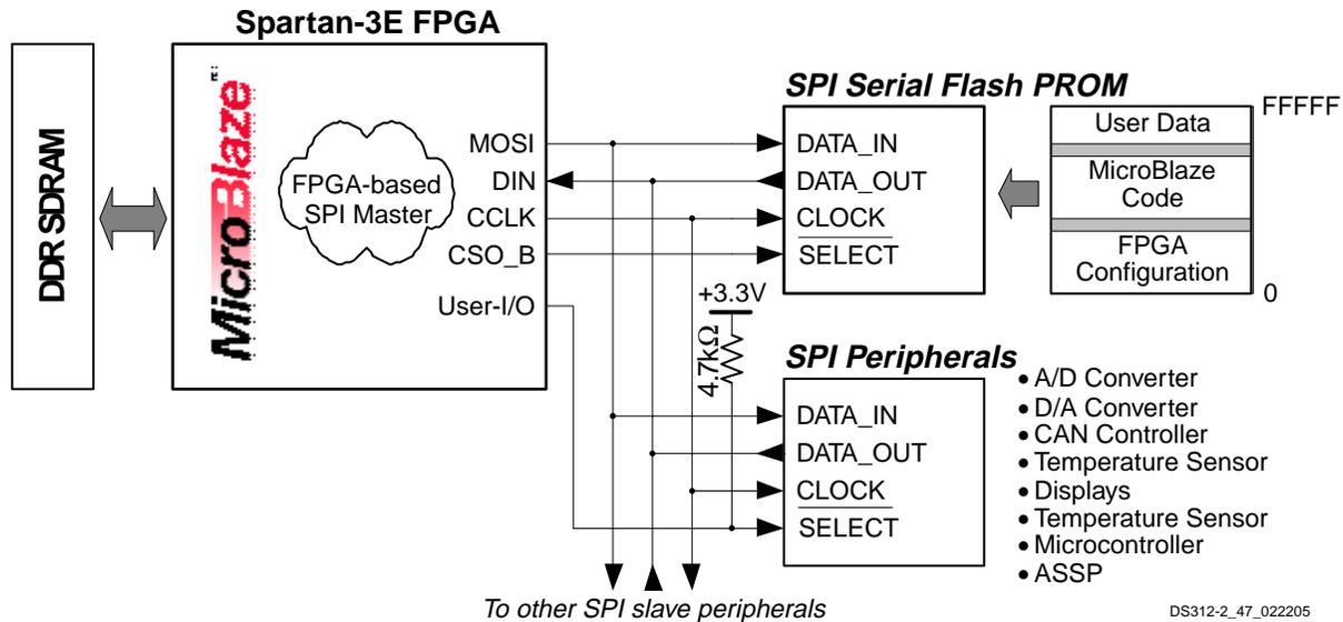
Figure 53: Using the SPI Flash Interface After Configuration
