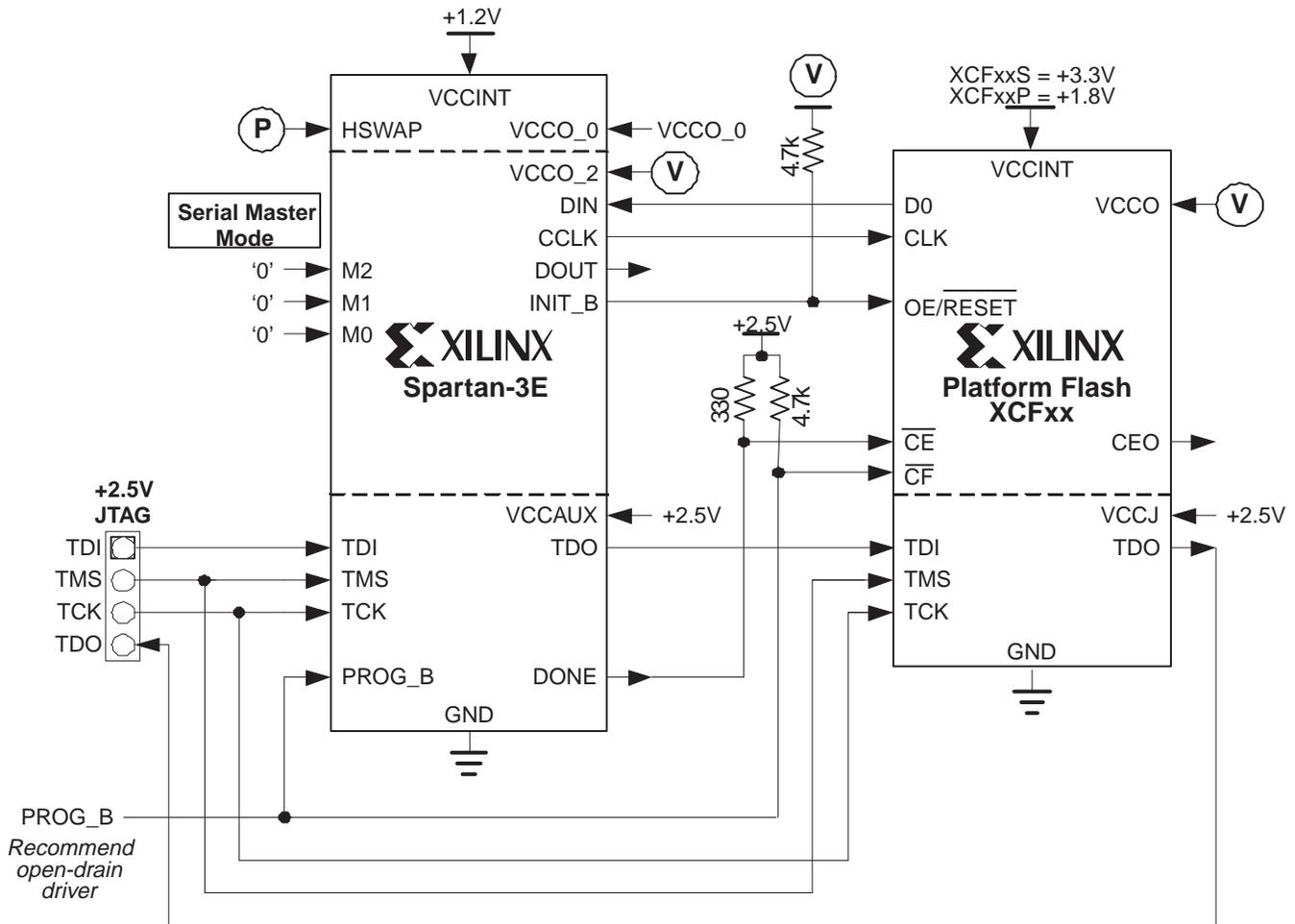
Figure 48: Master Serial Mode using Platform Flash PROM
