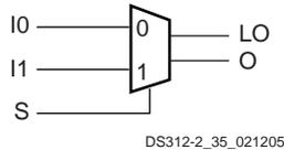
Figure 18: F5MUX with Local and General Outputs
