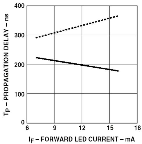
Figure 11. Propagation Delay vs. I<sub>F</sub>.
