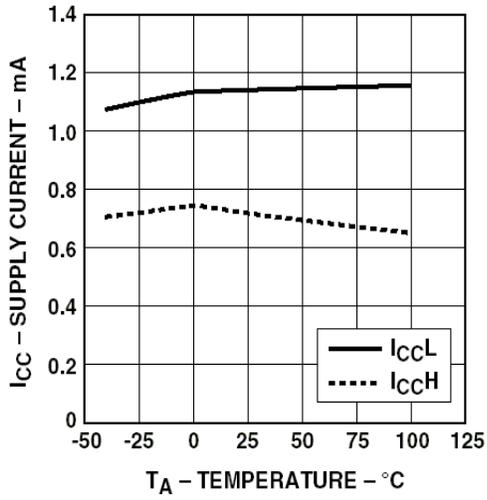
Figure 7. I<sub>CC</sub> vs. Temperature.
