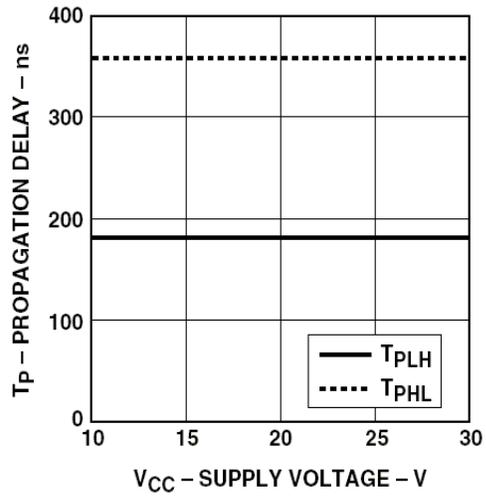
Figure 10. Propagation Delay vs. V<sub>CC</sub>.
