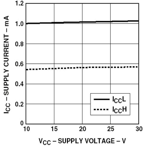
Figure 8. I<sub>CC</sub> vs. V<sub>CC</sub>.
