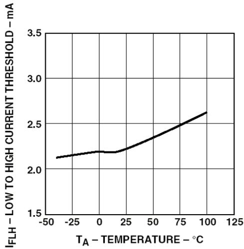
Figure 9. I<sub>FLH</sub> vs. Temperature.
