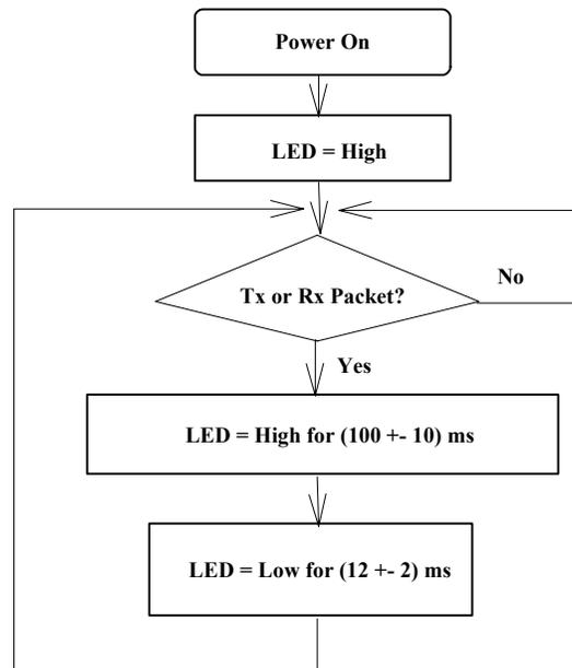
Figure 5. LED\_TX+LED\_RX
