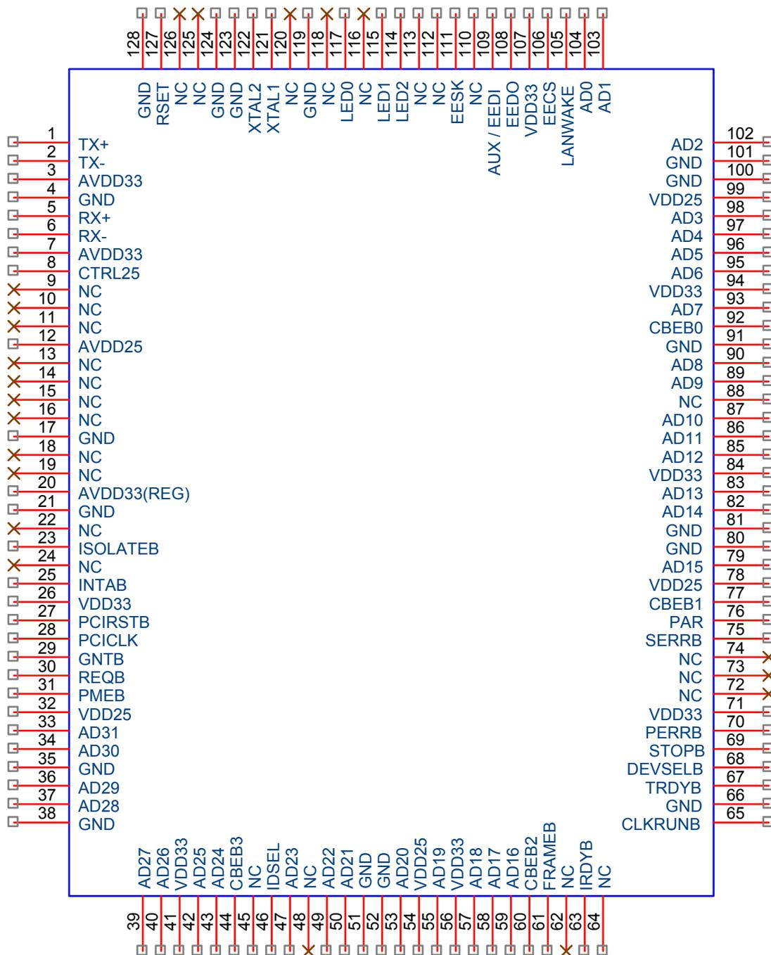
Figure 2. Pin Assignments
