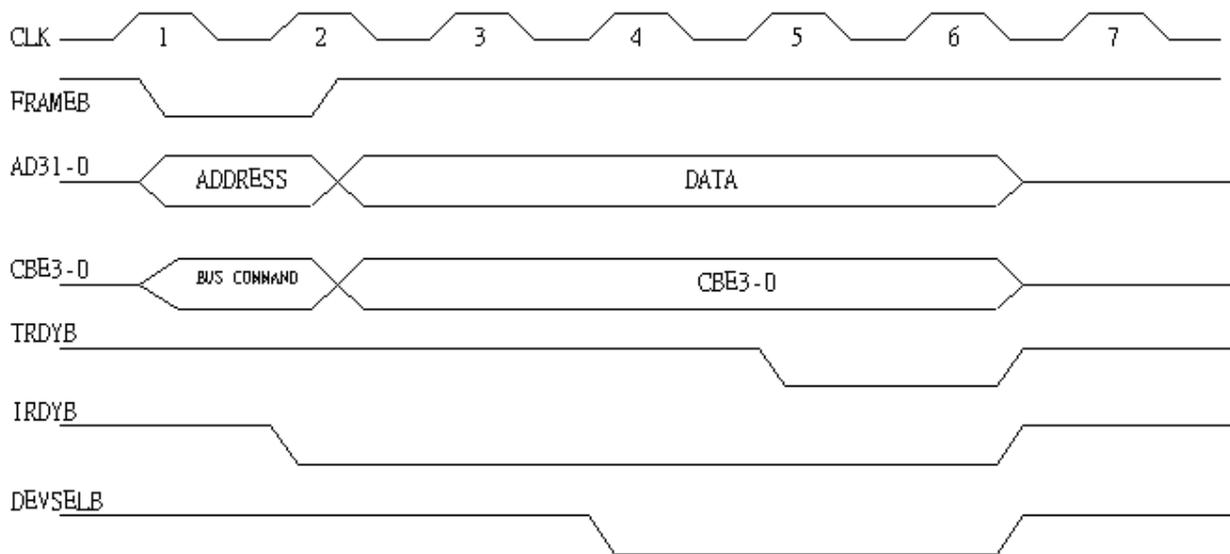
**Figure 7. Target Write**
