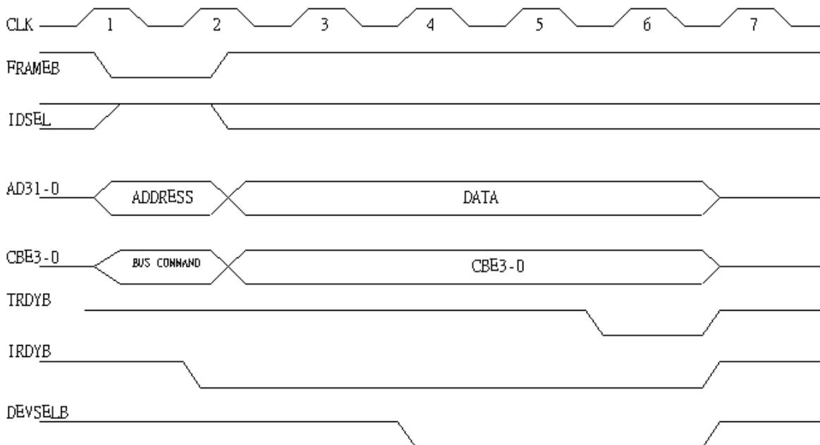
**Figure 9. Configuration Write**
