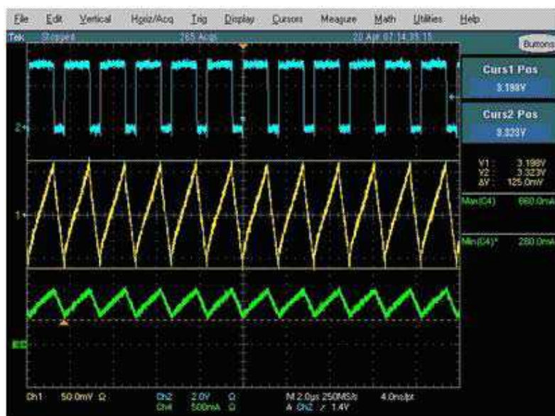
Figure 21. Electrolytic 100 \mu F (Ripple Too High)
