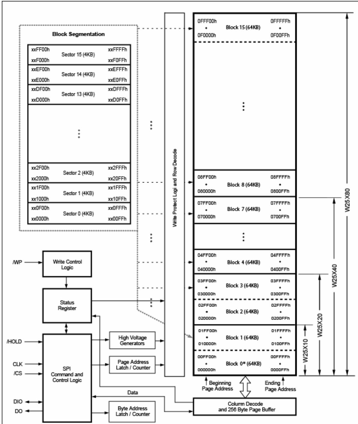
Figure 2. W25X10, W25X20, W25X40 and W25X80 Block Diagram
