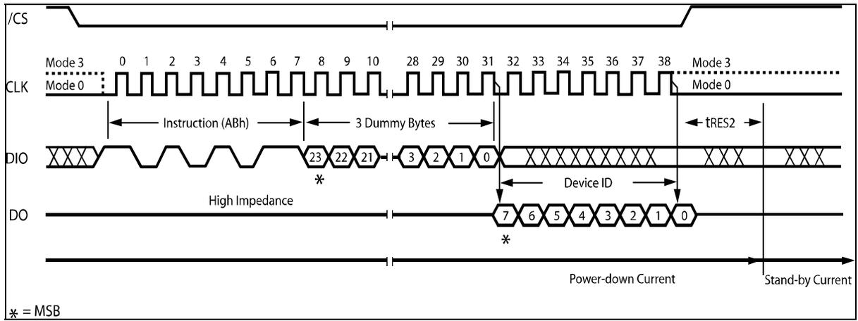
Figure 17. Release Power-down / Device ID Instruction Sequence Diagram
