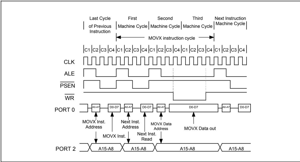
Figure 9: Data Memory Write with Stretch Value = 1
