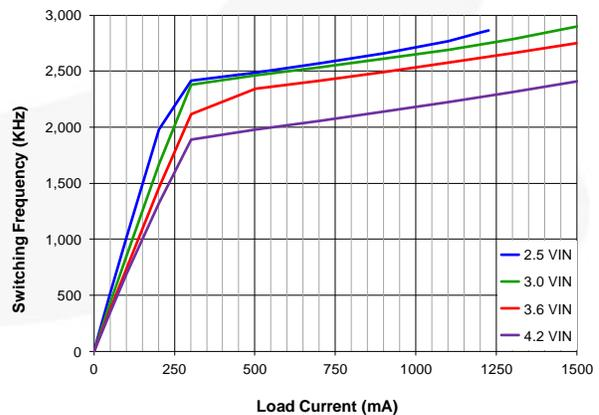
**Figure 16. Frequency vs. Load Current and Input Voltage**
