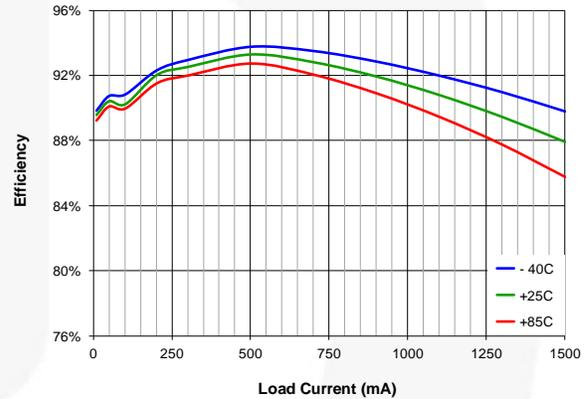
Figure 8. Efficiency vs. Load Current and Temperature
