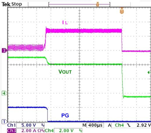
Figure 19. Overload Protection
