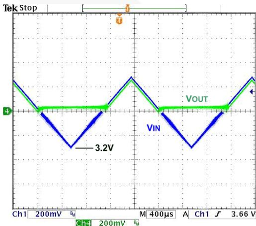
Figure 27. Bypass Entry / Exit, Slow  $V_{IN}$  Ramp 1 ms Edge, 500 mA Load,  $V_{OUT}=3.5\text{ V}$ , 3.2 - 3.8  $V_{IN}$
