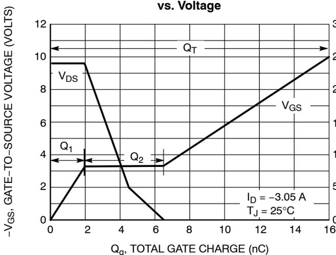
**Figure 9. Gate-to-Source and Drain-to-Source Voltage vs. Total Charge**
