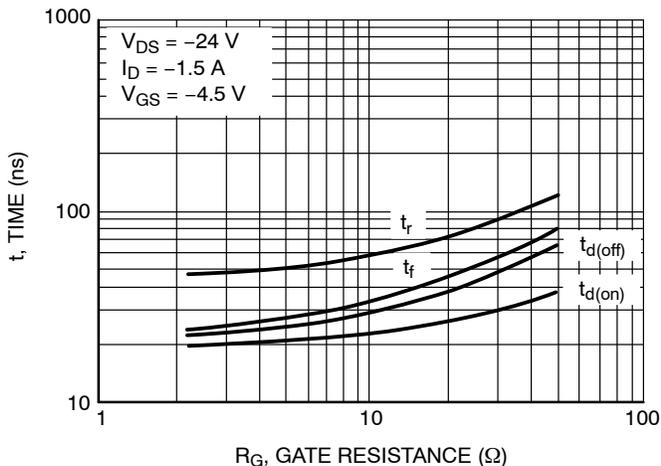
**Figure 11. Resistive Switching Time Variation vs. Gate Resistance**
