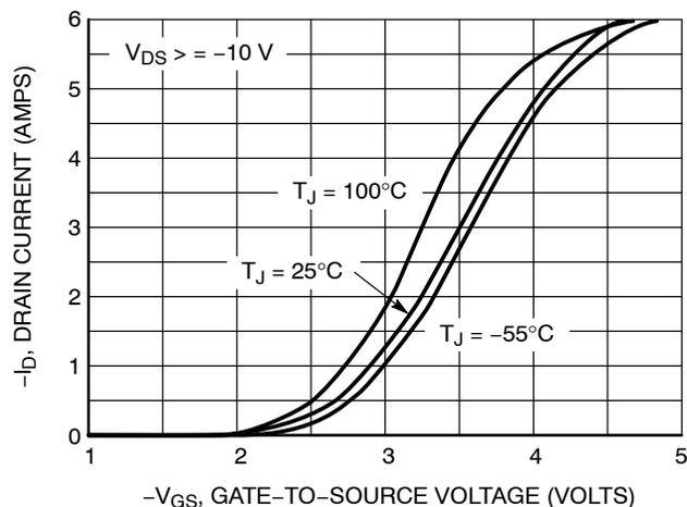
Figure 2. Transfer Characteristics
