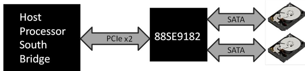
Fig 2. Typical Two Disk Application Example of 88SE9182
